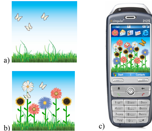
Figure 1. UbiFit Garden's glanceable display. a) at the beginning of the week—small butterflies indicate recent goal attainments; the absence of flowers means no activity this week; b) a garden with workout variety; c) the display on a mobile phone—the large butterfly indicates this week's goal was met.
