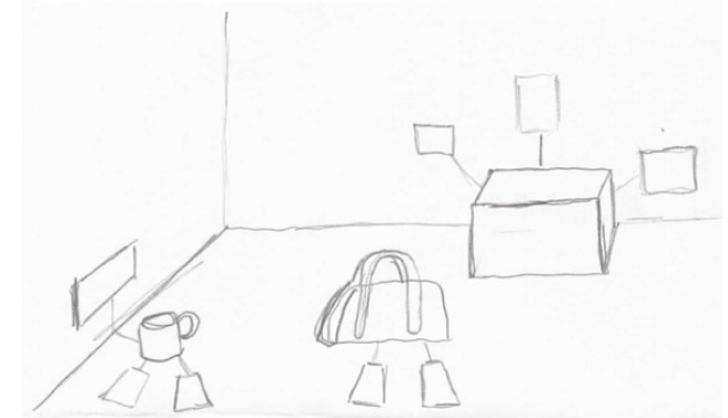
Figure 4: Physical objects with annotations. Annotations are anchored to an object and will display in the area surrounding it when viewed with a projector
