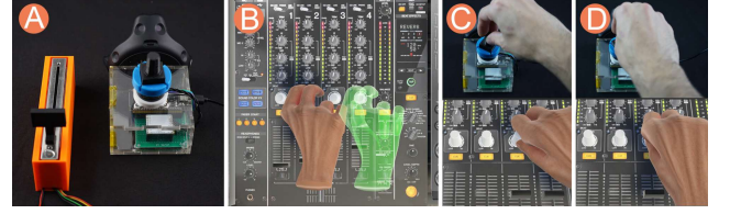
Figure 9: (A) displaying Feick et al. [21]’s slider proxy next to our knob proxy. (B) shows a user’s hand is redirected. (C) indicates the start position, while (D) shows the position of the hand after rotation in the real and virtual world.
