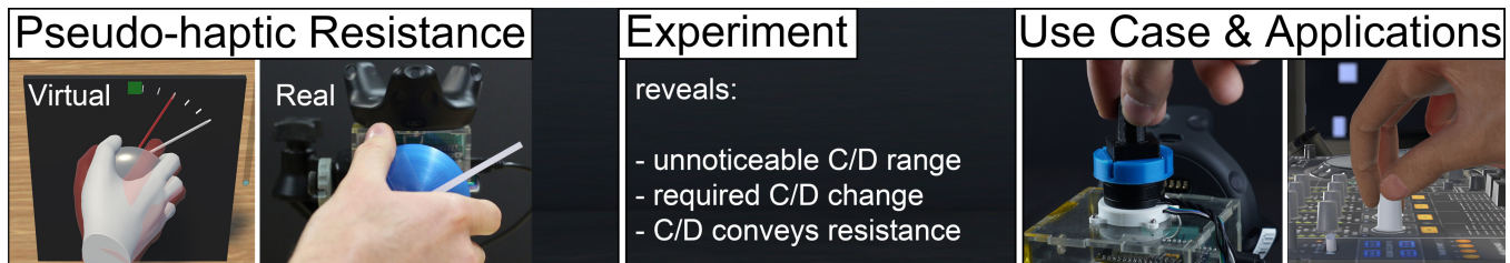
Figure 1: Pseudo-Haptic Resistance can be created by ‘slowing down’ a user’s real-world rotations of a knob. As a result the red needle rotates slower than the white needle.
