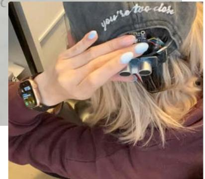
Version 2 of HACKLES attempted to fix the issues found with version 1. First, we moved the ranger to the back of a hat to limit false positives. We added padding to the choker to push the vibration motors against the skin. This version improved on version 1, but the ranger would still trigger for walls, trees and cars.
