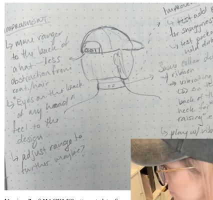
Version 2 of HACKLES attempted to fix the issues found with version 1. First, we moved the ranger to the back of a hat to limit false positives. We added padding to the choker to push the vibration motors against the skin. This version improved on version 1, but the ranger would still trigger for walls, trees and cars.
