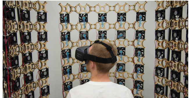
Figure 1. WindyWall is a 3-panel array for simulating wind.
