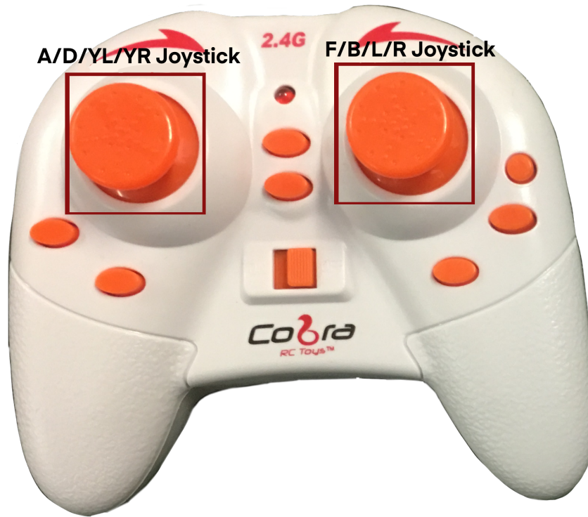
Figure 3.1: RC drone controller with its joysticks labeled. A/D/YL/RR controls the ascension, descension, and left and right yaw. F/B/L/R controls the drone's forward, backward, left, and right movement.
