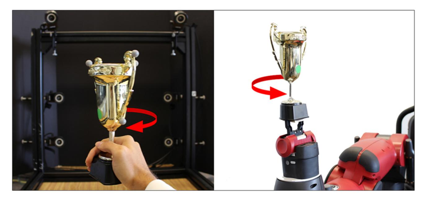
The robot's movement trajectory does not match the human motion due to the "wrist" joint limitation of the robot
