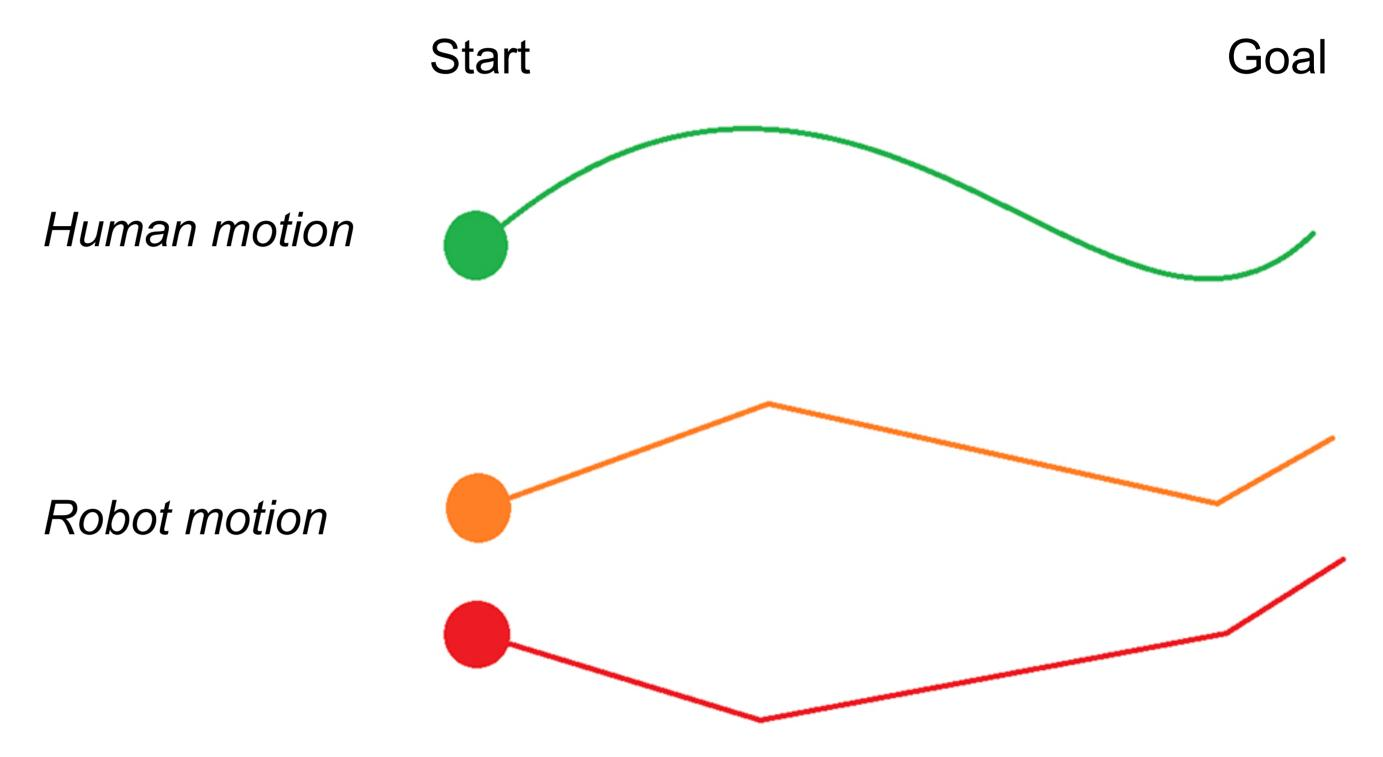
Human motion trajectory (top - green) compared to a similar robot motion (middle - orange), and a purely functional movement (bottom - red)
