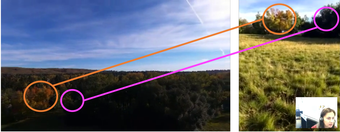
Figure 5.1: Two synchronized views into the same activity space. If the two views are from different perspectives, matching information between the two views is not always trivial. The annotations indicate the same objects appearing in the two views.
