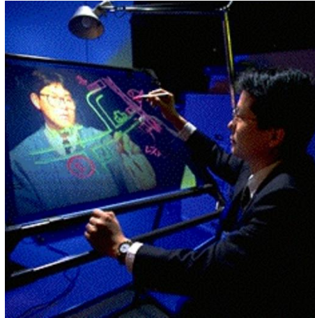
Figure 2.2. ClearBoard from Ishii et. al (1993), a shared workspace allowing remote coworkers to draw while maintaining eye contact and using natural gestures.
