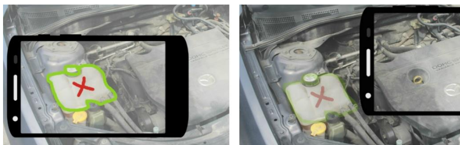
Figure 1.4. Stabilized annotations, attached to the objects of the scene in spite of the camera movement. Left: annotations are visible through the camera. Right: worker has moved the phone to right. Annotations are still anchored to the objects despite not being visible in the camera.
