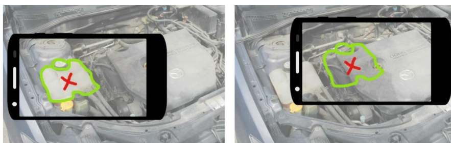
Figure 1.5. Non-stabilized annotations, drawn on top of the video feed, moving with the camera movement.
