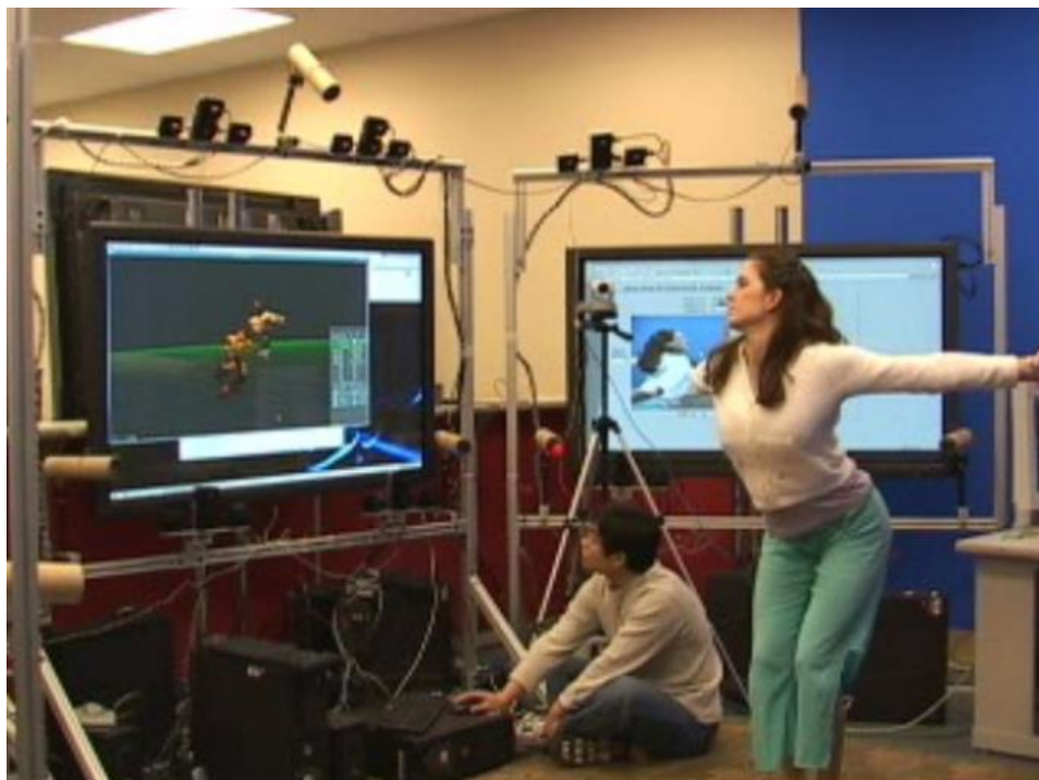
Figure 2.7 - Yang et al. (2006) presented a tele-immersive dancing system in which remotely located professional dancers' performance was recorded using 3D cameras and presented to them in a shared 3D space.
