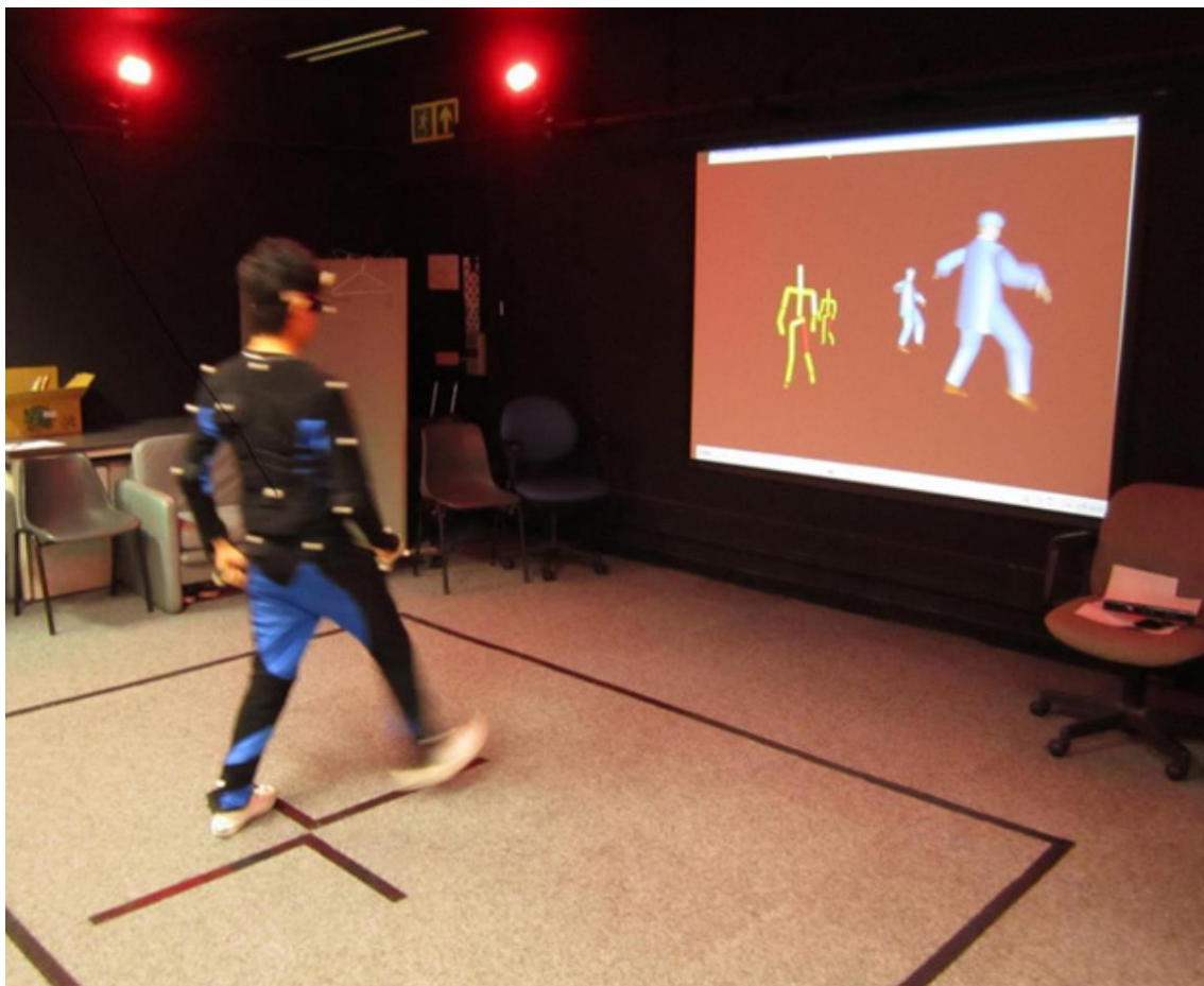
Figure 2.5 - DL-BUS (Yang et al. 2013) uses a 3D avatar to teach dancing to the learner based on the learner's movements which are tracked using a motion capture system.
