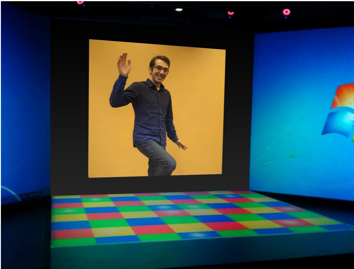
Figure 4.1 - LightFloor . In this system, the dancer stands in front of a large display in which they see their dancing partner. The dance floor is used to provide the dancer with dancing directions.
