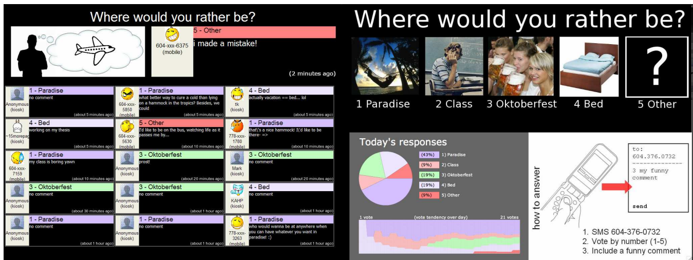
Figure 2. The MAGICBoard’s two displays have different functions. The right display is intended to be viewed from a distance, and functions as the “overview.” The left display is the “detail” display, and intended to be viewed up close.
