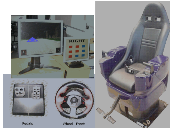
Figure 1: Apparatus for experiments: Kawada JoyChair R1 (right), LogiTech steering wheel and foot pedals that were attached to JoyChair (bottom), one monitor showing oval track, lead car and gauges, and other monitor showing distracter task (top, left).
